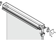
**02** If chain operated, fit the chain guide/s to the bottom of the transition plates using the screws provided.
