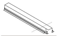
Insert the transition plates into the top grooves of the Headbox (Ensure they are the correct way round)
